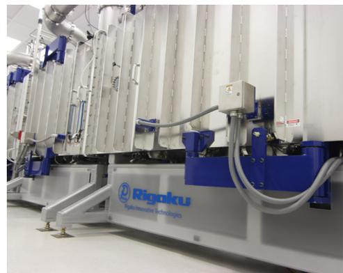
Rigaku Innovative Technologies' new large format in-line coating system. Developed specifically for EUV optics.
